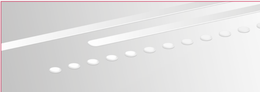
Glue application: dot and bead mode
