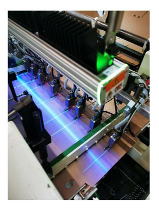
To support manufacturers of complex folding cartons, Baumer hhs has developed a new linear lighting system with high-power LEDs that accelerates job changeovers on folder-gluers by several minutes. Thanks to its uniform, very bright lighting, the system helps to reliably verify quality even at high machine speeds.
