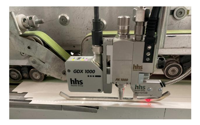
Testing the new PX 1000 cold glue head and new GDX 1000 cold glue monitoring sensor from Baumer hhs at the WestRock plant in Düren delivered proof positive: The new equipment once again significantly increases the reliability of adhesive application and therefore of the overall production process.
