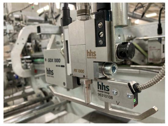
We are committed to achieving the highest quality in adhesive application. Our goal is to prevent waste by ensuring quality rather than just controlling it. Our PX 1000 adhesive application valve has already shown significant improvement by reducing contamination and gluing errors compared to the previous model, resulting in fewer rejects and resource savings. We are dedicated to continuously improving application quality and extending these improvements to other areas.
