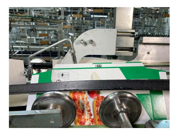
The Baumer hhs Side Seam Gluing Solution is a successful example of implementation. This solution replaces traditional wheel applicators with a nozzle applicator. During development, the main challenge was to ensure that the gluing flap was glued from start to finish. This was achieved through a new control process. The nozzle application solution of the Side Seam Gluing Solution allows for adhesive savings and reduces CO2 emissions associated with adhesive consumption by up to 50%. It also
