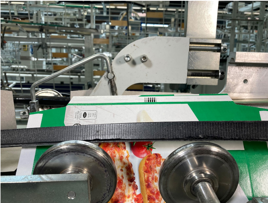
Figure 4 Efficient Longitudinal Seam Gluing with Side Seam Gluing Solution and Stitching Process
