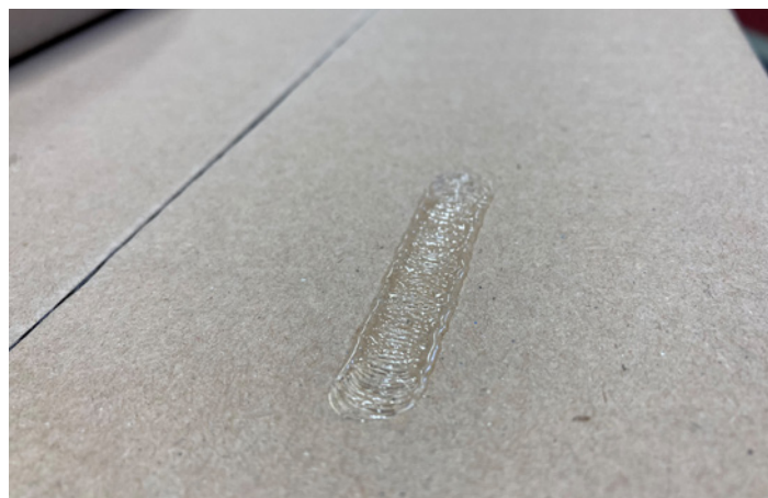
Spiral application for securing pallet loads.
