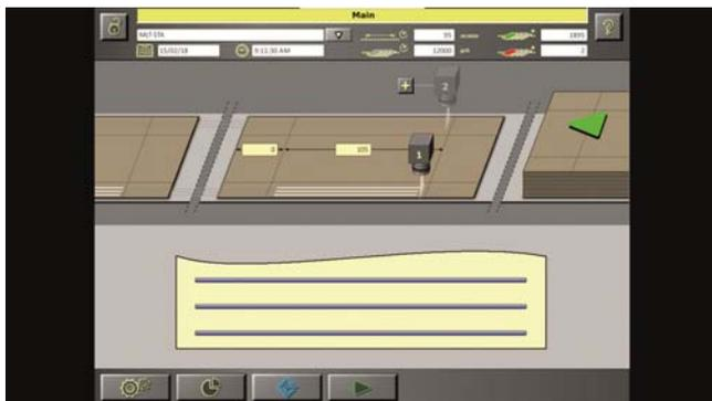
The MLT-STA is easy and convenient to set up and operate via touch screen. This low-cost control system checks glue application on one or two sides using MLT-40 optical, multi-bead cold glue sensors from Baumer hhs, which have proven their worth in practice for years the world over.
