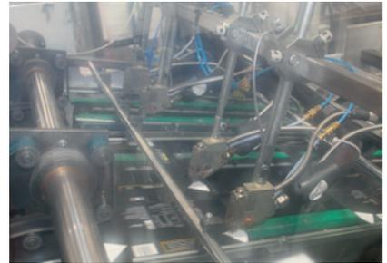
Even the tray former works with hot melt application systems from Baumer hhs.
