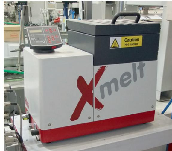
The hot melt heads are supplied by Xmelt hot melt units, which are very energy efficient in liquefying the adhesive granules and pumping the glue through heated hoses to the application heads.
